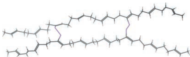
Fig. 1 Graphical representation of a unimodal polybutadiene network cross-linked using only sulfur atoms
